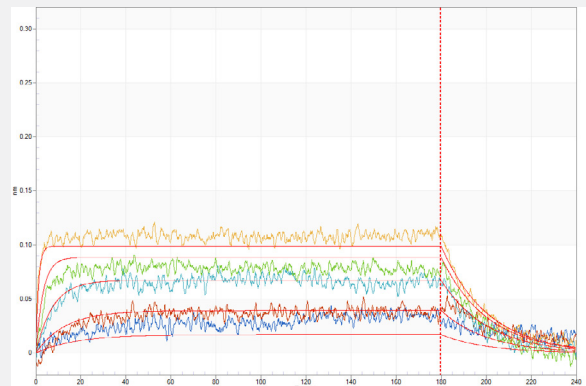
Comparison of furosemide (330 Da) binding onto carbonic anhydrase loaded Gator® SMAP vs competitor BLI.
